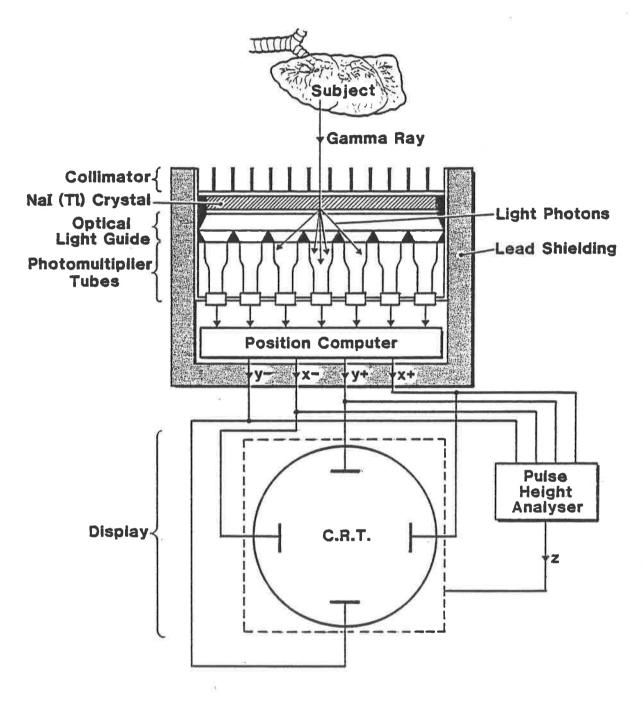
Fig. 4.10 Anger-Type Gamma Camera
